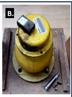
B - Hladinomer Robotron ( ^{60}\text{Co} , ^{137}\text{Cs} )
